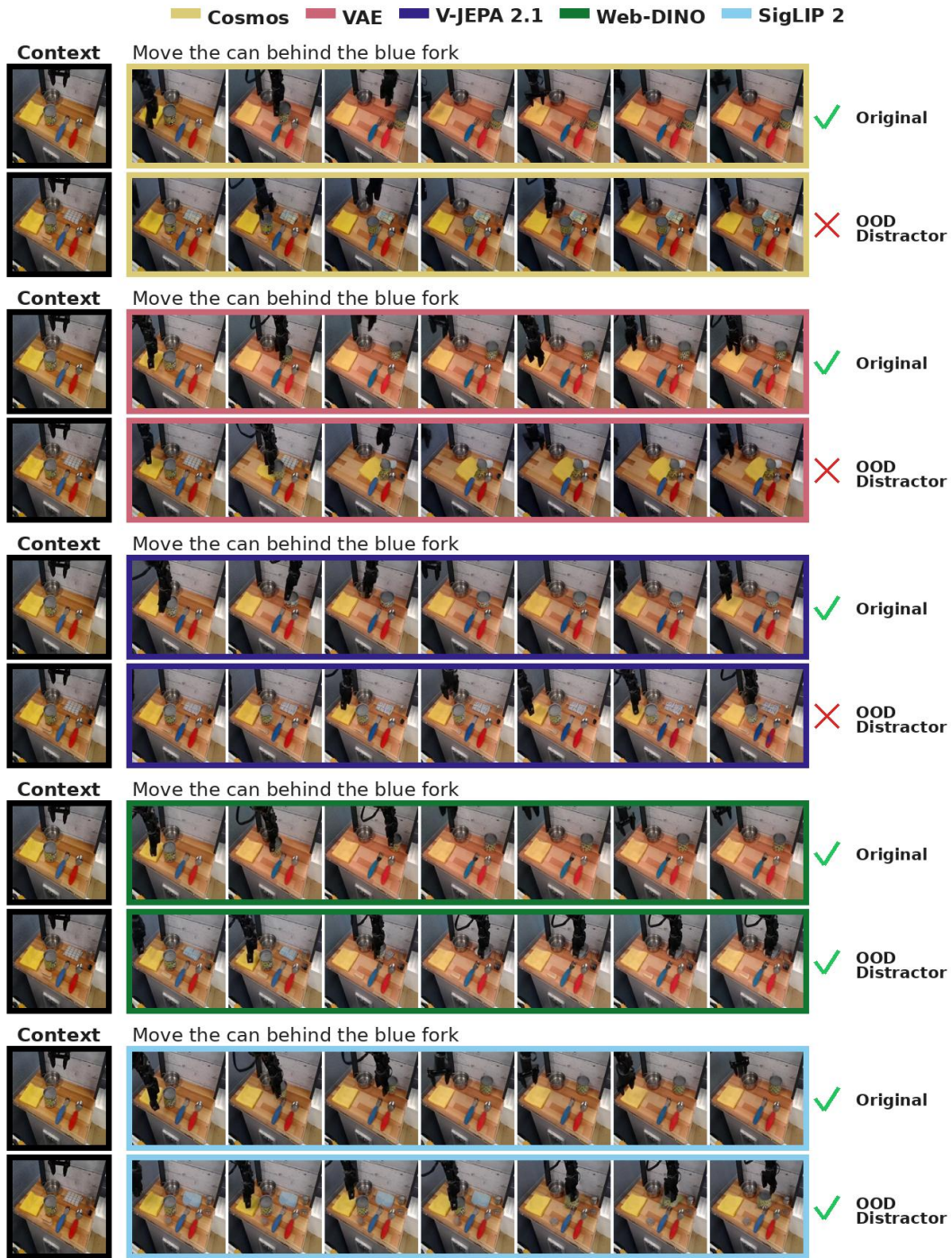
Figure 15: OOD Distractor comparison for the same episode: OOD distractor competes with the target objects and exposes whether a model can keep the target objects bound to the instruction. ✓ and ✗ show trajectories marked as success and failure by InternVL 3.5. Here, irrespective of the task success, the added object visually changes the predicted interaction for all models: the robot/can motion becomes less task-directed, the cans position is less consistently moved behind the blue fork, and the models appear to let the distractor alter the scene dynamics.
