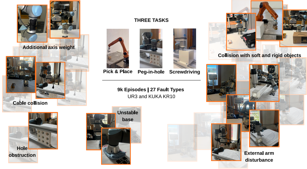
Figure 2: FactoryWave tasks and fault catalogue. Photographs of the robotic platforms (UR3, KUKA KR10) executing the three tasks (pick-and-place, peg-in-hole, screwdriving) and a representative subset of the 27 systematically injected fault conditions.
